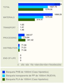
The LCA to go tool was used in order to define main environmental improvement strategies for polypropylene trays, aimed at the minimization of its carbon footprint.
